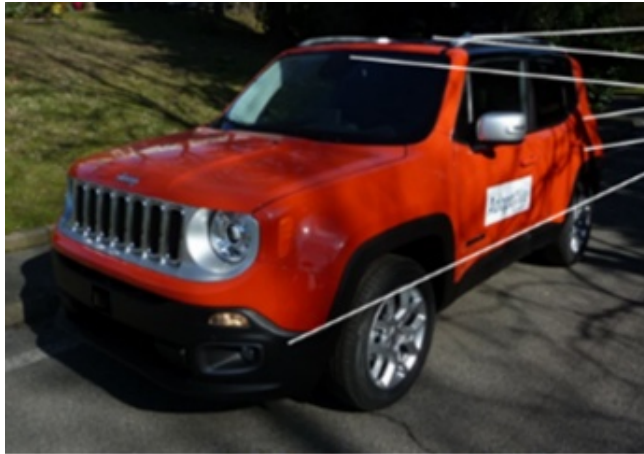
V2X antenna GNSS antenna Front RaCam Electronic Horizon Rear blind-spot Radar Side Ultrasound
